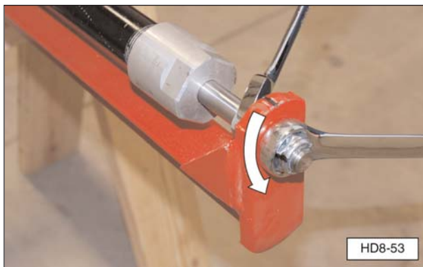
Loosen Lock Nut (C4) 1/2 Turn After Tightening.
