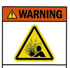
Hydraulic system parts and connections can contain high pressures which, if suddenly and unexpectedly released, can cause serious injury or death.
