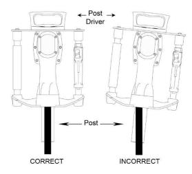
Figure 1: Post driver level example
