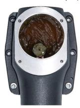
Figure 4: New grease example (before any single use)
