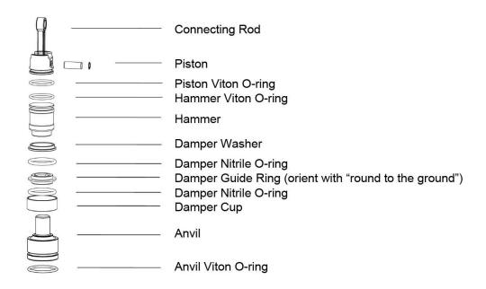
Figure 9: View of the orientation of internal parts
